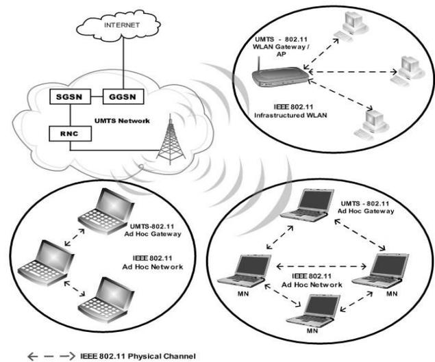
Figure 1: Architecture of Heterogeneous Wireless Network System
