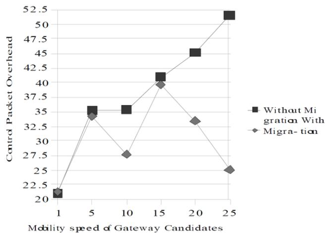
Figure 6: Effect of Mobile Gateway Migration on Control Packet Overhead with multiple sources
