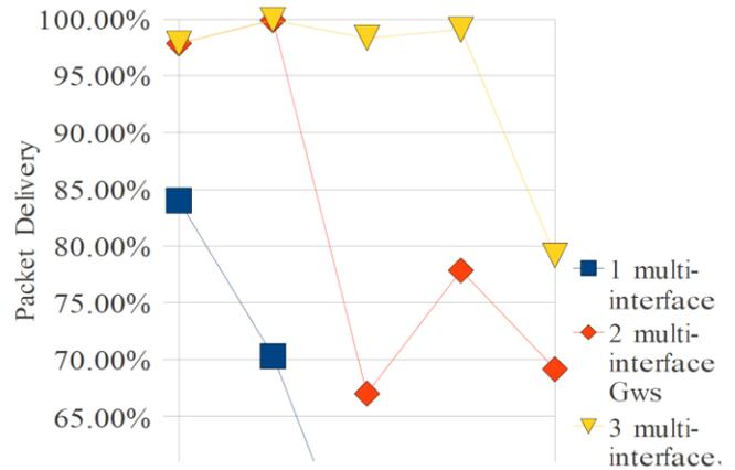
Figure 2: No. of sources (Vs) Data Packet Delivery Ratio with constant number of multi-interfaced Gateway Candidates
