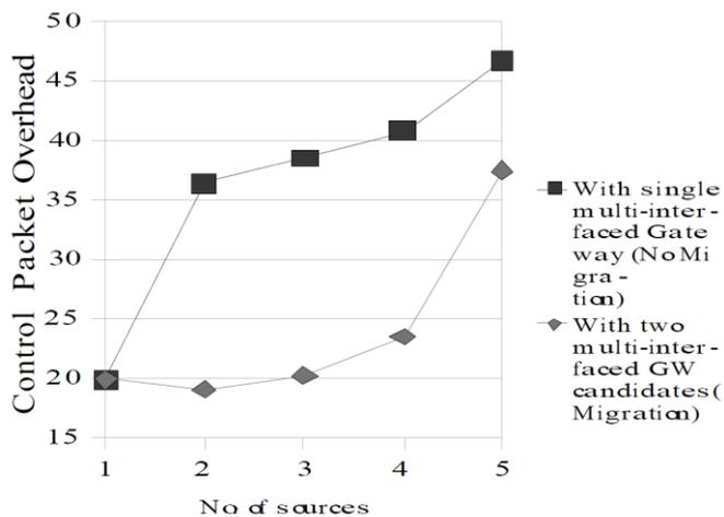
Figure 5: Effect of no. of sources on Control Packet Overhead
