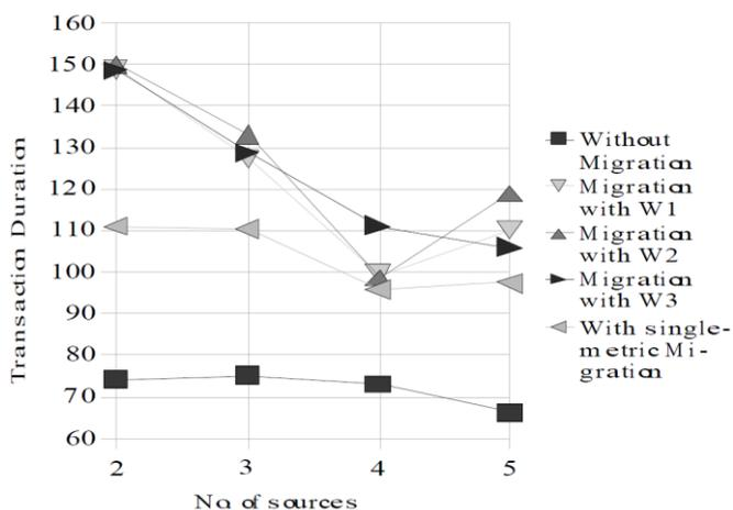
Figure 11: Effect of Multi-metric Gateway Migration on Transaction Duration against number of MANET sources
