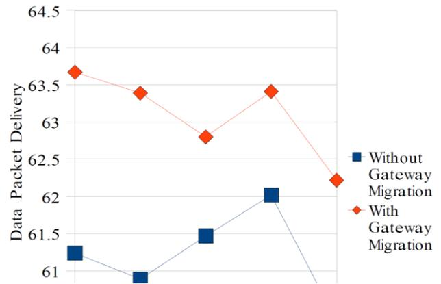
Figure 3: Effect of Migration of Mobile Gateways on Data Packet Delivery Ratio
