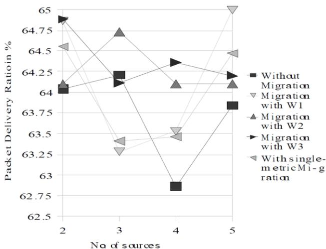
Figure 12: Effect of multi-metric Gateway Migration on Packet Delivery Ratio
