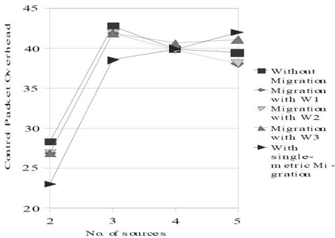
Figure 13: Effect of multi-metric Gateway Migration on Control Packet Overhead
