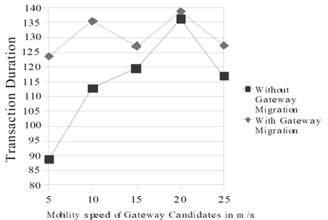
Figure 4: Effect of Mobile Gateway Migration on Transaction Duration with multiple sources
