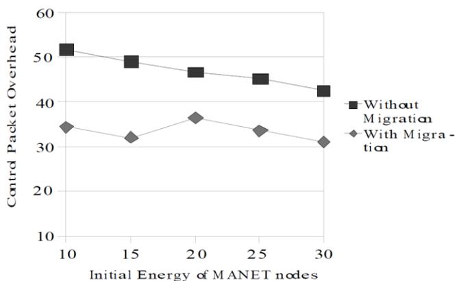
Figure 8: Effect of Energy-efficient Gateway Migration on Control Packet Overhead against initial energy of Gateway Candidates
