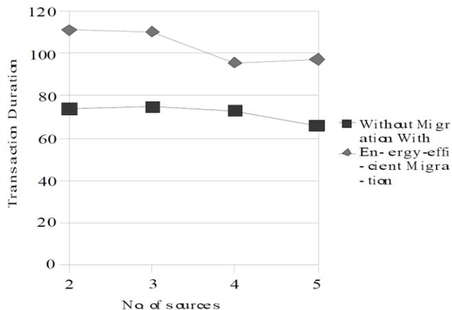
Figure 10: Effect of Energy-efficient Gateway Migration Transaction Duration against number of MANET sources
