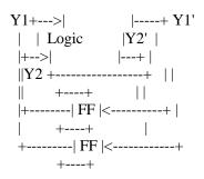
The set of FF's is a register, for example, and the combinational logic might be the adder. (I have left off all the ...'s that should be in here - obviously there can be more than just 2 inputs and 2 outputs.)
