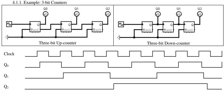
Timing Diagram for Three-bit Up-counter
