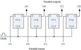
3.2. Shift Register = a register that accepts and/or transfers information serially.
