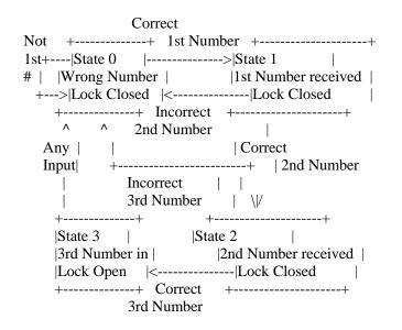
This State Transition diagram describes the behavior of the machine. Remember, State implies memory. We get to a given state based on a pattern of inputs. In digital design, memory = FF's. So we get to a given state based on the state we are currently in and the inputs at this time.
